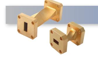
The HASCO WR-28 Millimeter Waveguide 90° Twist **HWTW28-2-ES** operates from 26.5 GHz to 40 GHz. This WR-28, Ka-Band waveguide 90° twist is constructed with a Square UG-599/U Flange.
