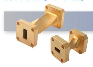
The HASCO WR-34 Millimeter Waveguide 90° Twist **HWTW34-1-ES** operates from 22 GHz to 33 GHz. This WR-34, waveguide 90° twist is constructed with a Square UG-595/U-M Flange.
