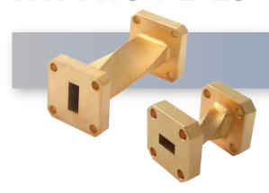
The HASCO WR-34 Millimeter Waveguide 90° Twist **HWTW34-2-ES** operates from 22 GHz to 33 GHz. This WR-34, waveguide 90° twist is constructed with a Square UG-595/U-M Flange.
