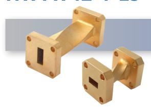
The HASCO WR-42 Millimeter Waveguide 90° Twist **HWTW42-1-ES** operates from 18 GHz to 26.5 GHz. This WR-42, K-Band waveguide 90° twist is constructed with a Square UG-595/U Flange.
