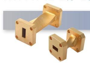
The HASCO WR-42 Millimeter Waveguide 90° Twist **HWTW42-2.5-ES** operates from 18 GHz to 26.5 GHz. This WR-42, K-Band waveguide 90° twist is constructed with a Square UG-595/U Flange.
