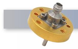
The HASCO HWCA-101F-EL waveguide to coaxial adapter is manufactured for end-launch (straight) requirements. This adapter is designed for WR-10 waveguide and has a UG387/U-MOD compatible flange with a 1.0mm Female connector. A 1.0mm Male version is also available upon request.
