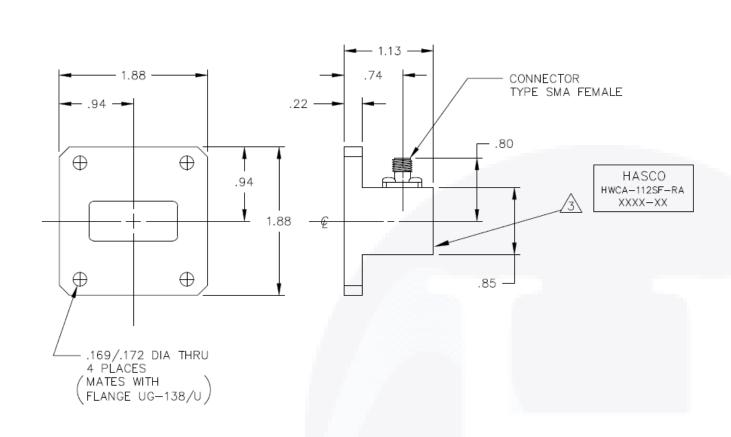
To view online, go to: <a href="https://www.hasco-inc.com/adapters/adapters-waveguide/wr-112-to-sma-female-waveguide-to-coax-adapter-right-angle-design-7-05-ghz-to-10-ghz-ug138-u-flange/">https://www.hasco-inc.com/adapters/adapters-waveguide/wr-112-to-sma-female-waveguide-to-coax-adapter-right-angle-design-7-05-ghz-to-10-ghz-ug138-u-flange/</a>
