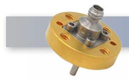
The HASCO HWCA-121F-EL waveguide to coaxial adapter is manufactured for end-launch (straight) requirements. This adapter is designed for WR-12 waveguide and has a UG387/U compatible flange with a 1.0mm Female connector. A 1.0mm Male version is also available upon request.
