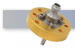
The HASCO HWCA-151F-EL waveguide to coaxial adapter is manufactured for end-launch (straight) requirements. This adapter is designed for WR-15 waveguide and has a UG385/U compatible flange with a 1.0mm Female connector. A 1.0mm Male version is also available upon request.
