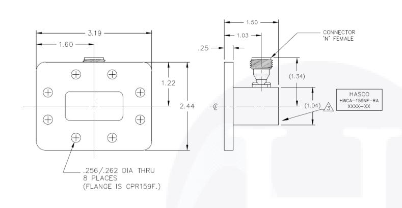
To view online, go to: <a href="https://www.hasco-inc.com/adapters/adapters-waveguide/wr-159-to-type-n-female-waveguide-to-coax-adapter-right-angle-design-4-9-ghz-to-7-05-ghz-cpr159f-flange/">https://www.hasco-inc.com/adapters/adapters-waveguide/wr-159-to-type-n-female-waveguide-to-coax-adapter-right-angle-design-4-9-ghz-to-7-05-ghz-cpr159f-flange/</a>
