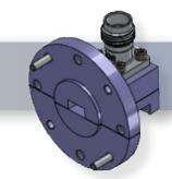
WR-19 to 1.85mm Female Precision Waveguide to Coax Adapter Right Angle Design, U-Band - 40 GHz to 60 GHz
