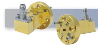
The HWCA-121F-RA is a precision WR-12 waveguide to 1.0mm coaxial adapter operating in E Band with a 60 GHz to 90 GHz frequency range. This adapter offers a robust design with Low VSWR and Low Insertion Loss with a UG-387/U flange.
