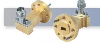
The HWCA-1518F-RAR is a general purpose WR-15 waveguide to 1.85mm coaxial adapter operating in V Band from 50 GHz to 67 GHz. This adapter is constructed with a UG-385/U flange.
